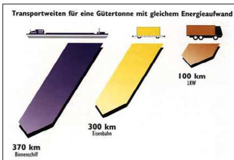
Picture 64 - Transport distances for 1 ton commodities with the same energy consumption
